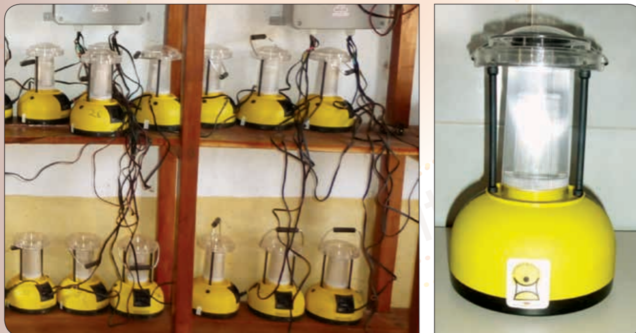
The LaBL lantern used at the Energy Centre
